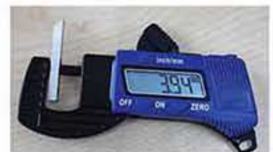
Workpiece thickness testing
